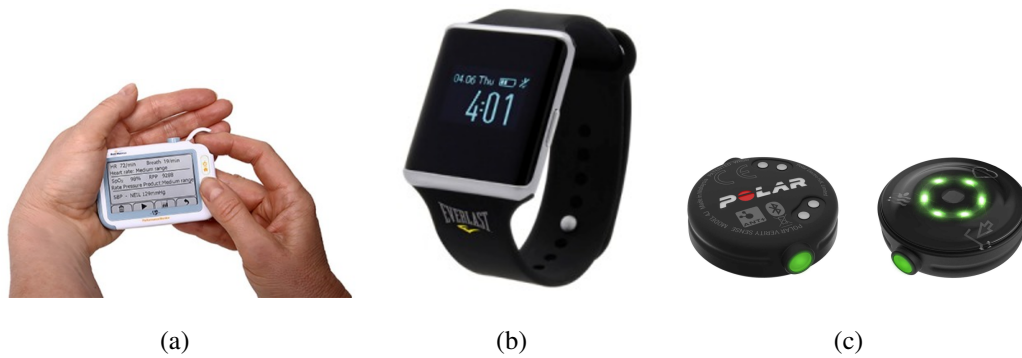
Figure 2.6: Various types of HR monitoring tools (Hahnen et al., 2020). (a) BodiMetrics Performance Monitor tricoder. Vital signs are measured by placing the right index finger on the plethysmography sensor located in the upper right corner beneath the flap. (b) Everlast smartwatch. Vital signs are measured by the electrodes and a photoplethysmography sensor located at the back plate. (c) Polar verity sense. Vital signs are measured by the electrodes and a photoplethysmography sensor located at the back plate.
